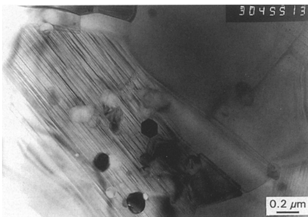
Figure 9 Transmission electron micrograph of the hot pressed \text{Si}_3\text{N}_4 (powder)-mullite (sol-gel) mixture, showing the presence of unreacted \text{Si}_3\text{N}_4 particles.
